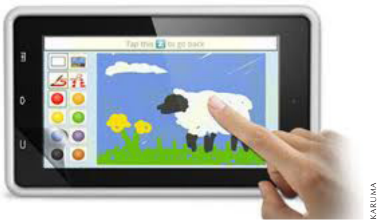
The PlayBase+ tablet for children has a glass touchscreen imbedded with silver ions to help reduce bacteria on the screen's surface.
