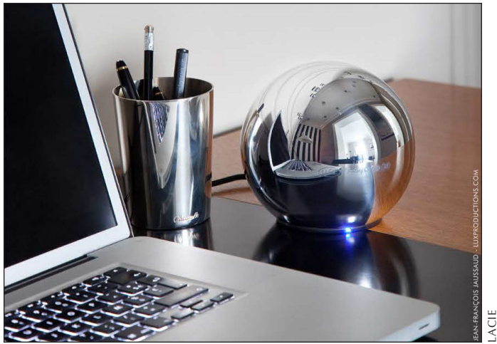
This handcrafted silver-plated sphere by LaCie contains a 1-terabyte hard drive.
