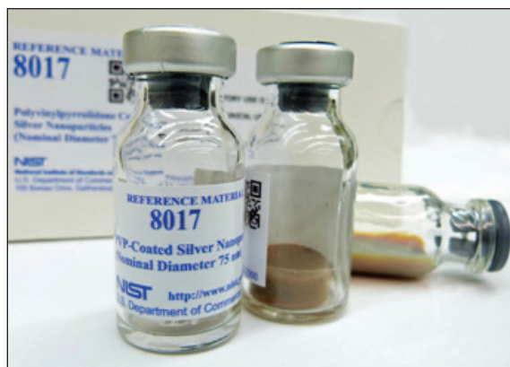
NIST's new silver nanoparticle reference material is designed for extended shelf life to support environmental health and safety studies.
