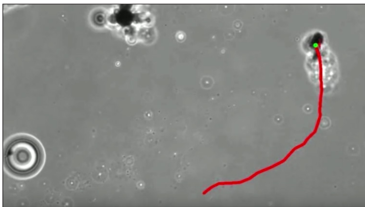
Microbots coated with silver kill germs as they travel through water. Click on image to view video.
