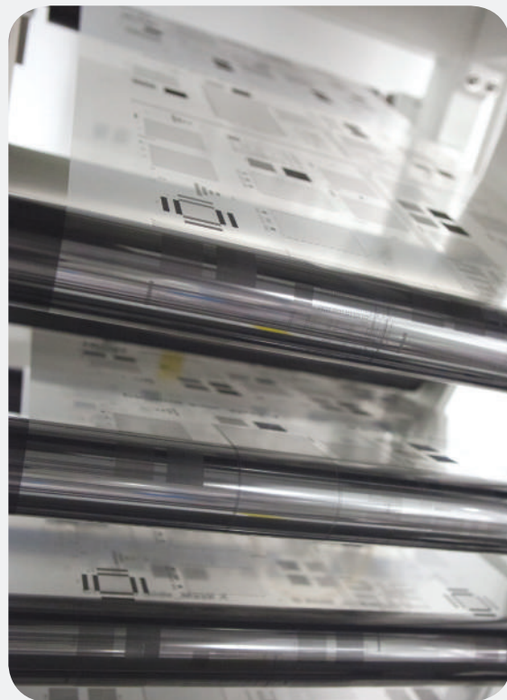
Image depicts silver metal touch sensors, which are used in cell phones and tablets. Photo provided courtesy of Kingsbury Corporation
