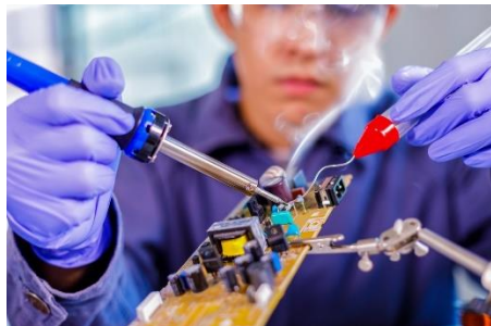
Soldering a component to a PCB
