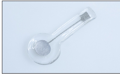
This all-hydrogel electrode containing silver flakes, used for electrocardiography (ECG), was 3D printed.
